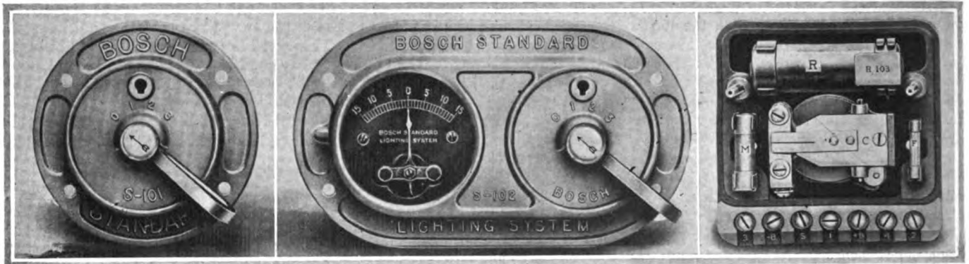
The switch of the new Bosch Standard lighting equipment combines an ammeter and full control for all circuits, while the switch can be locked. The cut-out, fuses and regulating ballast coil are in a separate box
